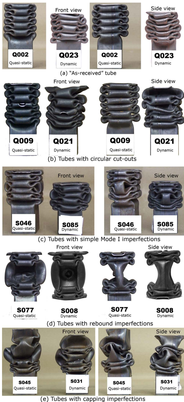
Fig. 31 Photograph showing the comparison between quasi-statically and dynamically crushed tubes
