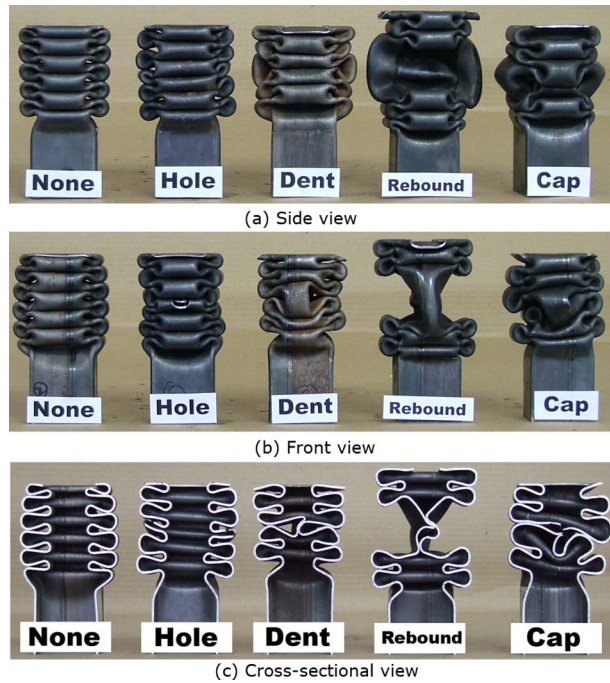
Fig. 17 Photograph showing square tubes with and without imperfections crushed quasistatically
