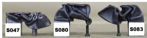
Fig. 23 Photograph showing tubes collapsing in unstable mode (bolts included for photographic purposes)
