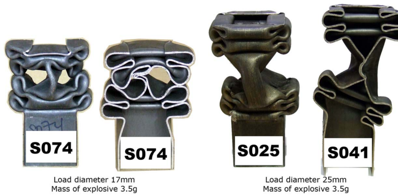
Fig. 15 Crushed 50 mm tubes with asymmetric blast response
