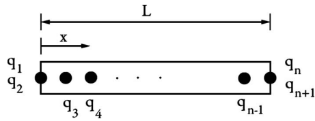
Fig. 3 Beam element used for p-version FEM
