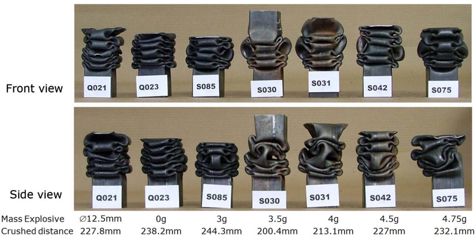
Fig. 29 Photographs showing dynamic axial crushed 50 mm square tubes with and without imperfections caused by an explosive of load diameter of 17 mm with a drop mass of 329 kg from a nominal height of 3.26 m (imperfections in tube Q021 are drilled holes)
