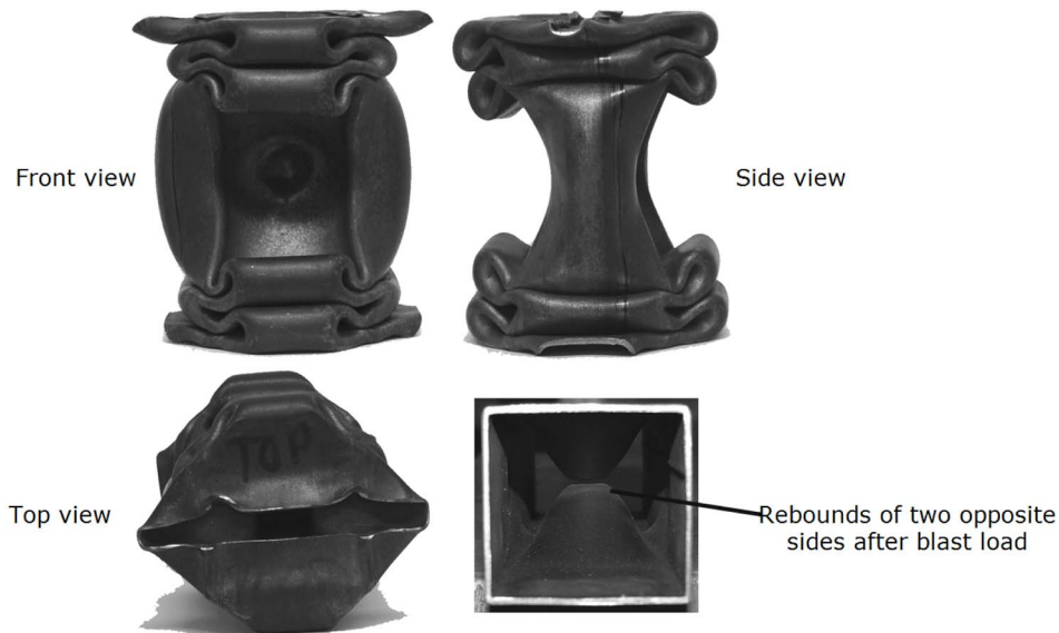
Fig. 26 Photographs showing the dynamic axially crushed blasted loaded 50 mm tube with a drop mass of 210 kg from a 4 m drop height (mass of explosive: 3.5 g, load diameter: 25 mm, crushed distance: 200 mm)
