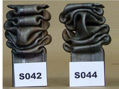
Fig. 27 Photographs showing the dynamic axial crushed 50 mm the square tubes with blast imperfection caused by a 4.5 g of PE4 at a load diameter of 17 mm (drop mass: 329 kg, nominal drop height: 3.26 m)
